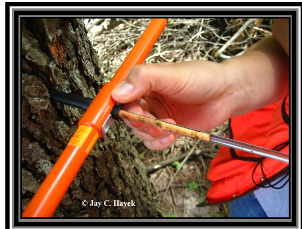
An increment core extracted from a black cherry tree using a Suunto™ increment borer.
